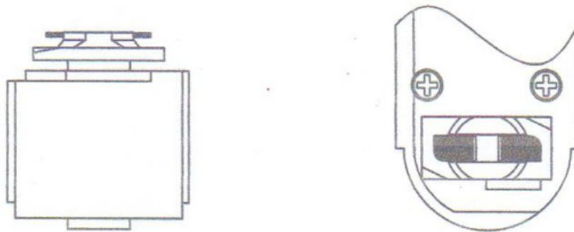
**3** HOW TO INSTALL THE TK-HEADS CORRECTLY. ENSURE THAT THE REBATE ON THE TK-HEAD HOUSING IS ALIGNED WITH THE ALIGNMENT RIB ON THE TK-TRACK. THEN ROTATE THE HOUSING IN THE CORRECT DIRECTION AND ENGAGE THE LOCKING MECHANISM.
