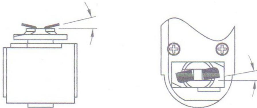
**2** RE-ALIGN & RE-SEAT CONTACTS WITH LONG NOSE PLIERS.
