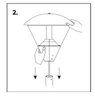
Place lantern head on top of pole or wall bracket.
