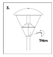
Fix the light to the pole or wall bracket FB3003.
