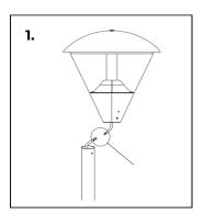
For a safe and correct installation, ensure a water tight connection between the supply cables.
