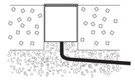
3. All fittings have a plastic mounting niche included. Please see chart below for preparing the cavity. The top of the niche should be below the level of the finished surface, correctly calculate the required height of the top of the niche to the finished surface. Extra cavity depth may be required below the niche for the IP cable connection.
