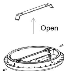
3. Fix mounting bracket to the ceiling or wall using suitable screws.
